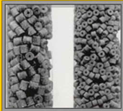
Sock Loading Method 100 mm tube
